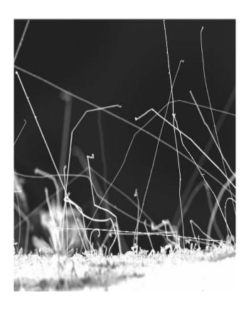
Zinc whiskers were first discovered in 1948 by Bell Labs when a "whisker" on a zinc-plated bracket caused increased losses in quartz filters used in a telephone transmission system superscript.
